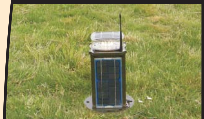
Emergency Runway Edge Lighting
